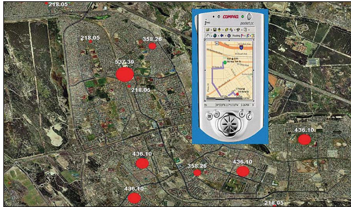
SAP is linked to GIS to extract monthly maintenance costs of water bursts in the Khayelitsha service area. Bursts have been captured with mobile GIS devices.
